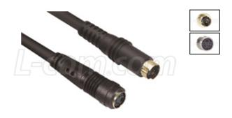
These high quality S-Video cable assemblies utilize dual 75 Ohm coaxial cables for unmatched video signal transmission. The molded strain relief Mini Din 4 connectors with gold plated contacts assure distortion free performance. We typically carry these exceptional quality cable assemblies in stock in 7 handy lengths from 1 to 20 ft.
